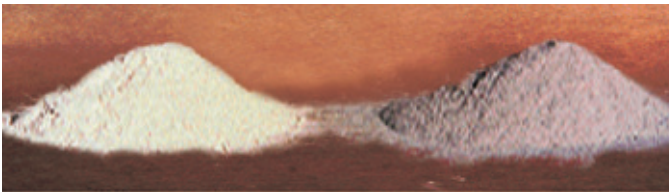
Figure 1-3. Typical ash colors.
